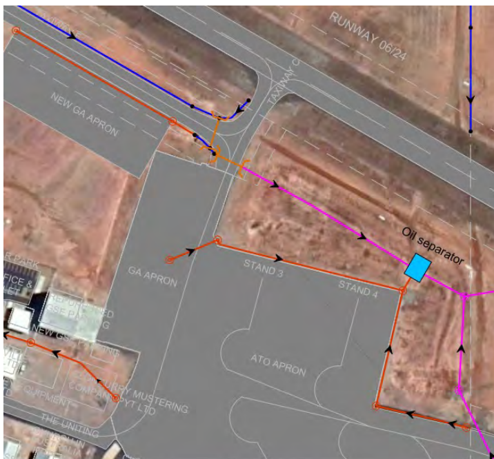
Figure 24 Oil separator to cater the flow for existing ATO apron and GA apron.
