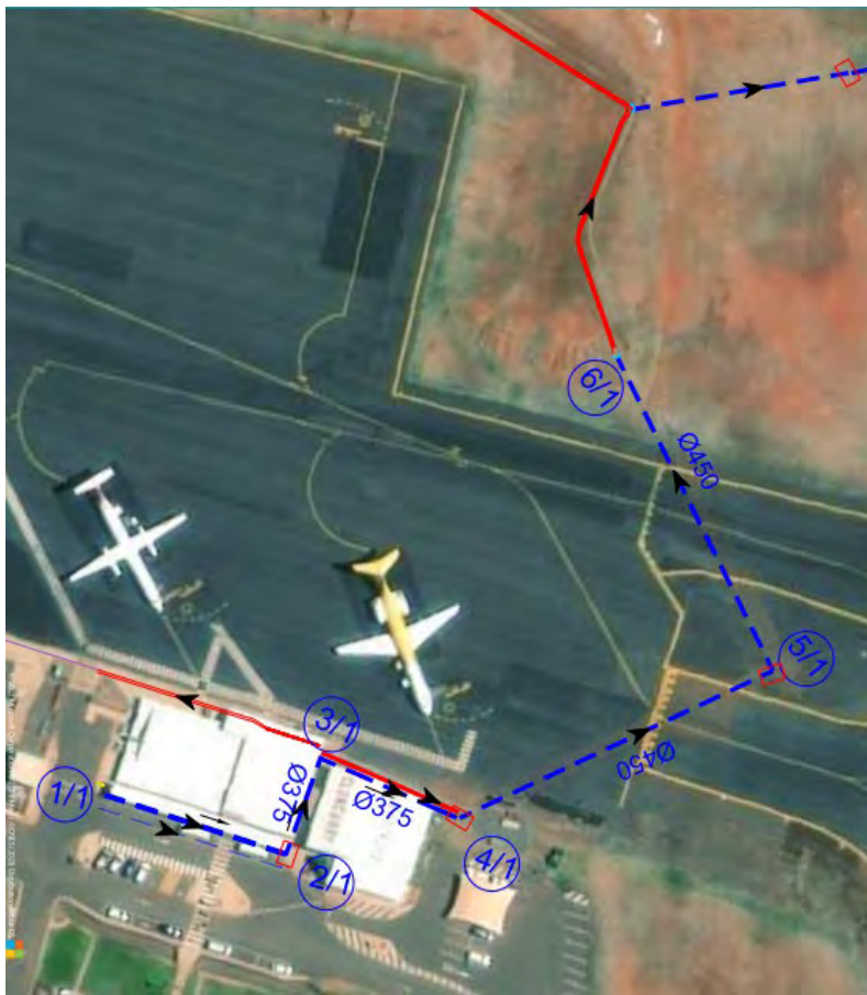
Figure 19 Existing Drainage Infrastructure for Existing Taxiways and Aprons
